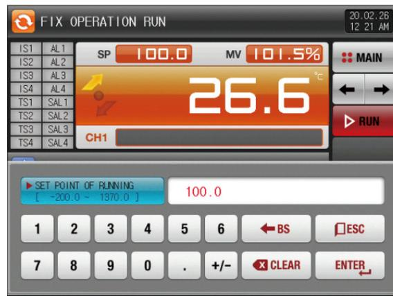
[Fig. 4-27] Screen for target value setting input key of program for stationary operation in program/stationary operation still screen (Non synchronized operation)
