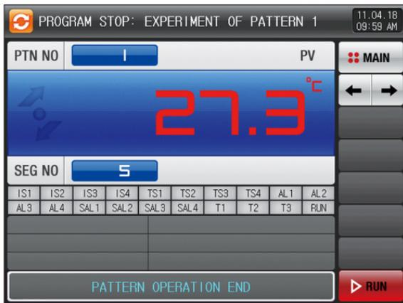
[Fig. 4-47] Termination screen for operation of program
