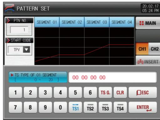
▲ The input key is displayed when 00 00 00 00 (Time signal) is touched by. The button **TS G** to set the sub output is appeared when **AUX** button on the right top is touched by.
