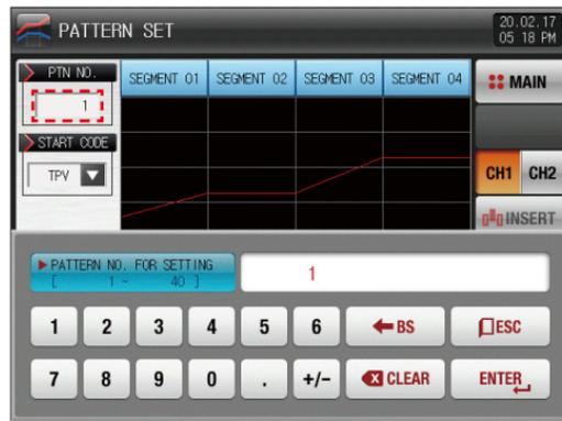
▲ The input key to set the pattern number is displayed when the "Pattern number" button is touched by.
