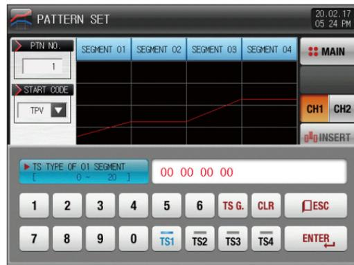
▲ The input key to set the time signal is displayed when 00 00 00 00 (Time signal) button is touched by. The time signal can be set for TSetting~TS8 when TS.G. button is touched by.
