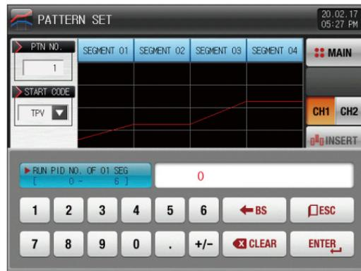
▲ The input key to set the segment PID is displayed when  (SEG PID) button is touched by.
