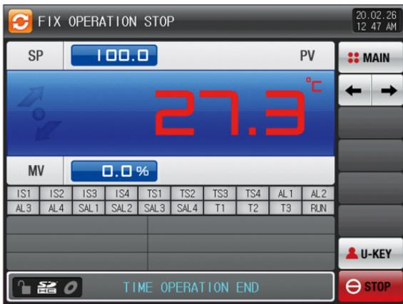
[Fig. 4-39] Termination screen for operation of stationary time setting (General)
