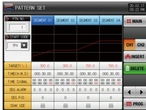
▶ **INSERT** , **DELETE** buttons are activated when **SEGMENT 01** button is activated.
