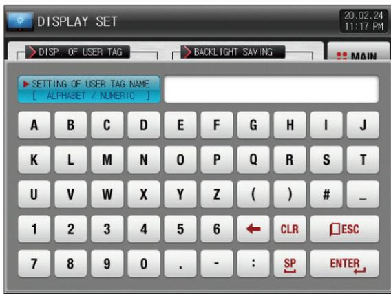
[Fig. 8-2] User tag name setting screen in channel1 and 2
