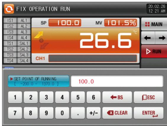
[Fig. 4-4] Screen for input key for setting target data of operation
