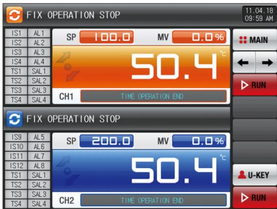
[Fig. 4-11] Termination screen for operation of stationary time setting (Non synchronized operation)
