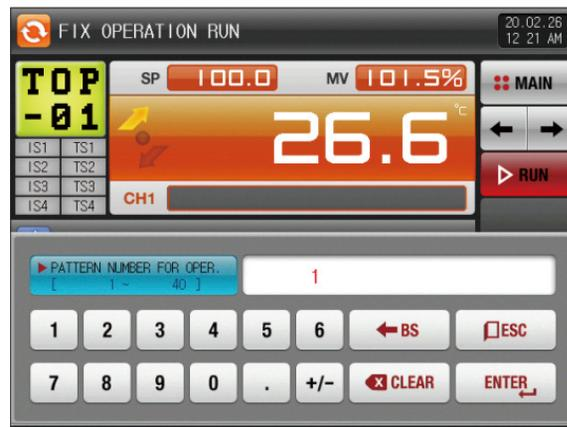
[Fig. 4-29] Screen for pattern number setting input key for program operation in program/stationary operation still screen (Synchronized operation)
