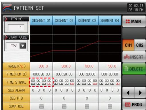
▲ It is a screen for sub output setting. Select the sub output in [4, Control & Transmitting output] in [Installation manual]. It is displayed in red in pattern edition screen and the sub output can be set.
