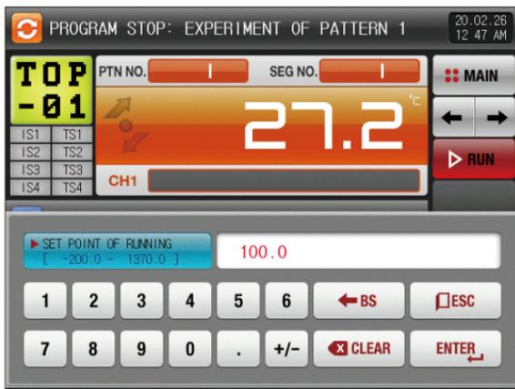
[Fig. 4-28] Screen for target value setting input key for stationary operation program/stationary operation still screen (Synchronized operation)
