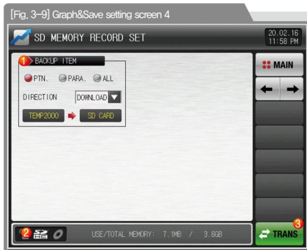
Setting the items and direction of transmitting in SD card and TEMP2000
