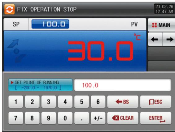
[Fig. 4-35] Screen for input key for setting target data of operation
