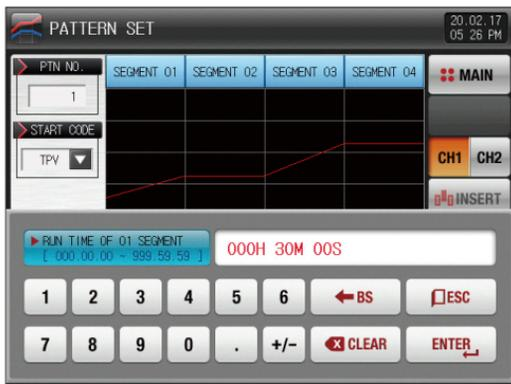
▲ The input key to set the segment time is displayed when 002.00.00 (Time) button is touched by.
