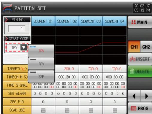
▶ When the "Starting condition" button is touched by, the input key to set the starting condition is displayed
