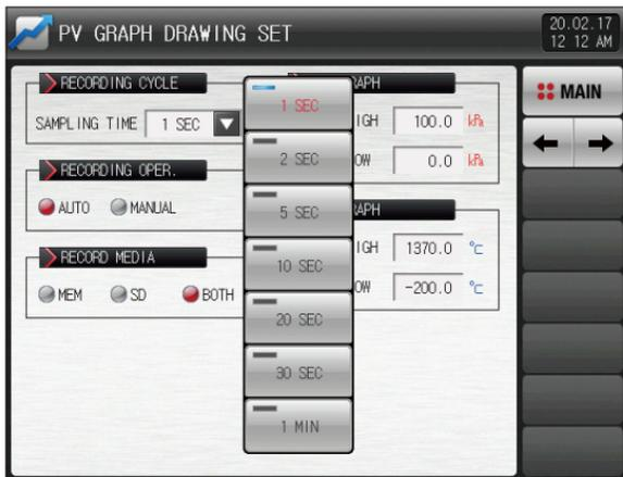
[Fig 3-11] Sampling time of Recording cycle setting screen
