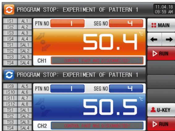
[Fig. 9-1] Control unit communication error screen
