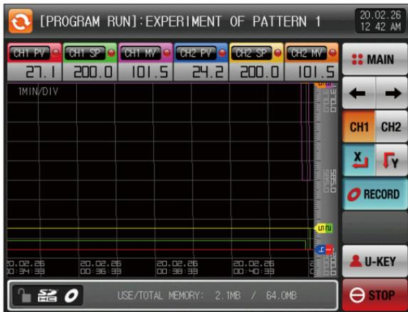
[Fig. 4-21] X-Axis setting screen of Program operation
