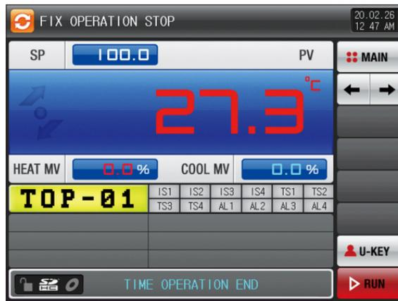
[Fig. 4-40] Termination screen for operation of stationary time setting (Heating · Cooling)
