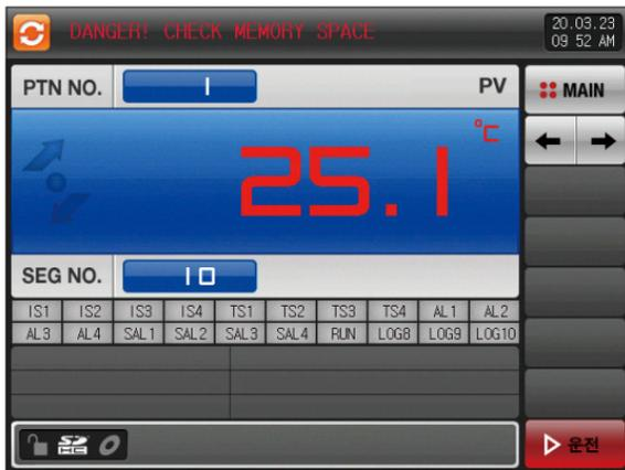
[Fig. 4-49] Screen for warning of shortage of memory capacity
