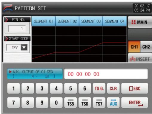
▲ The input key is displayed when  (Time signal) is touched by. The button **TS G.** to set the sub output is appeared when **AUX** button on the right top is touched by.
