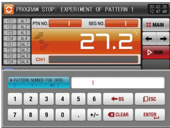
[Fig. 4-15] Screen for pattern number setting input key to be operated
