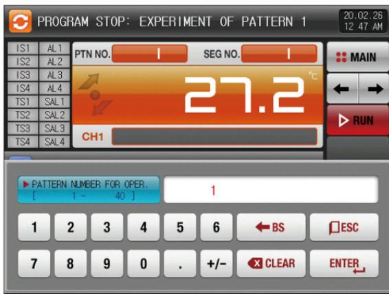
[Fig. 4-26] Screen for pattern number setting input key of program to be operated in program/stationary operation still screen (Non synchronized operation)
