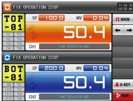
[Fig. 4-12] Termination screen for operation of stationary time setting (Synchronized operation)
