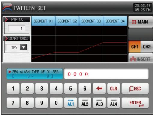
▲ The input key to set the segment alarm is displayed when  (SEG alarm) button is touched by.
