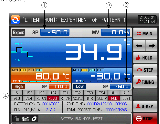
[Pic. 4-12] The 2nd operational screen for program operation (Low temperature room)
