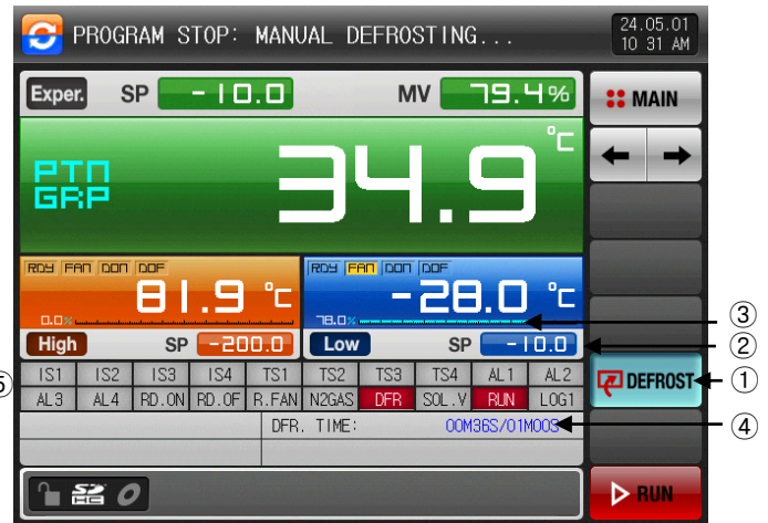
[Pic. 4-5] The 2nd manual defrosting
