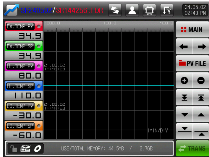
[Pic. 3-8] The second screen for graph & save (not select the graph display)
