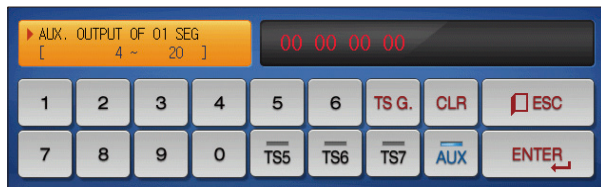
▲ Input key for sub output setting Refer to sub output in [4. Control & Transmitting output] in [Operation manual] for sub output setting.
